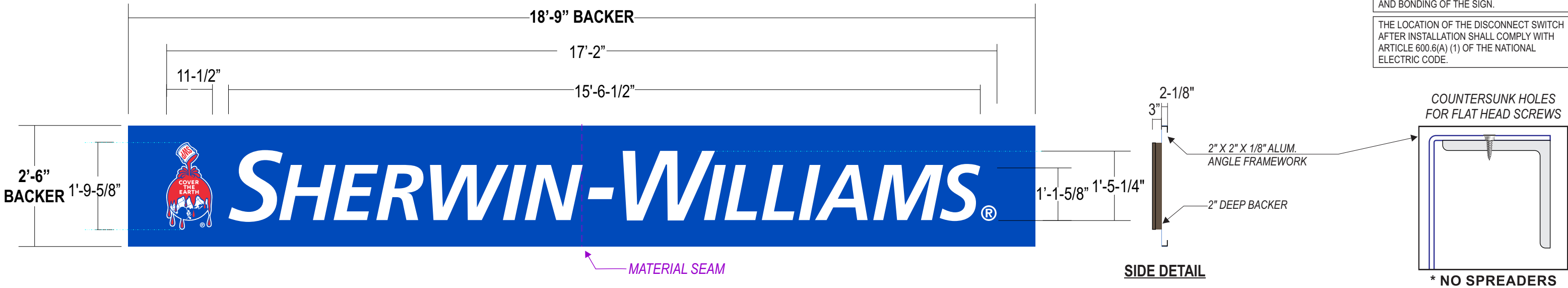
FACE LIT | RACEWAY| GENERIC INSTALL
